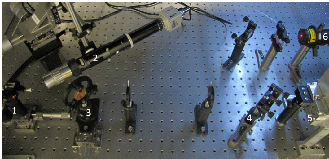
Figure 2.5: The photograph of the microdisk reflow set - up. (1) Sample holder, (2) Charge - Coupled Device camera, (3) ZnSe lens, (4) Flip mirror, (5) CO 2 laser and (6) He - Ne laser.
